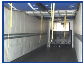
Split Bulkheads swing up & down, slide forward & back
